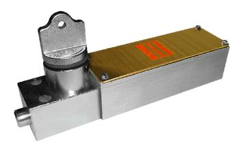
Type S Auxiliary Switches are slow-make, slow-break devices that respond directly to the movement of the lock bolt when the key is rotated. One, two, three or four sets of contacts are available. The Type S auxiliary switches can be furnished on the following interlocks:
